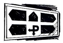
The driver receives advance notice of forthcoming turns from a panel mounted in the centre of the dash. For straight-ahead driving, the centre green arrow is illuminated. Should a right or left turn be needed, a warning buzz will alert the driver. An amber arrow will be illuminated one road before the turn is required, a red arrow will show that the turn is required on the next road available.
