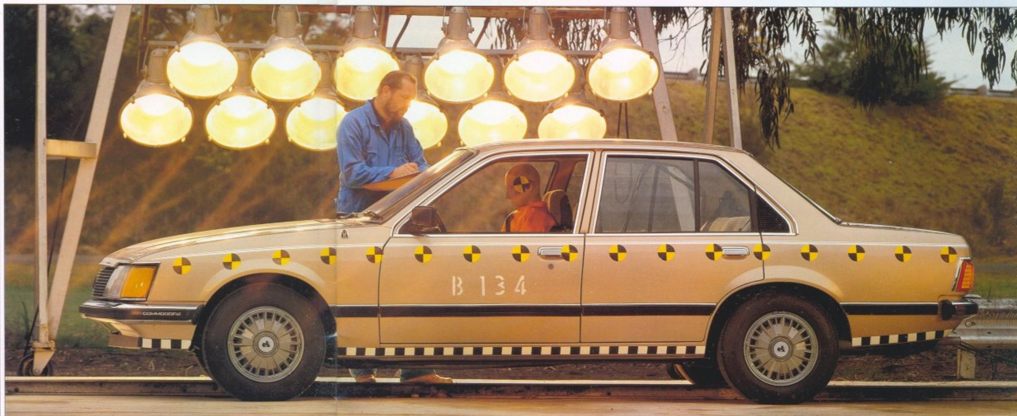
Left: Commodore's front body absorbs impact forces. The engine hood folds backward rather than penetrating the windscreen. Barrier impact testing under lights and cameras proves Commodore's passenger protection
