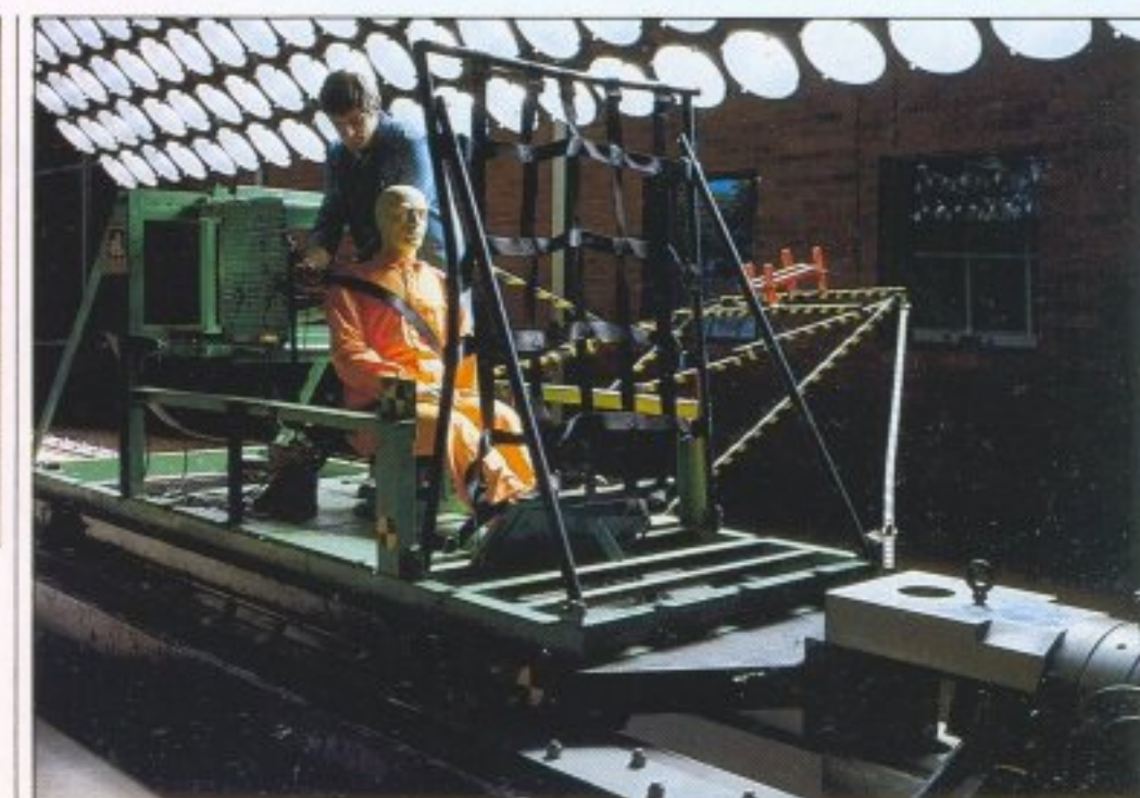
Above: Detail showing "child proof" rear door locks. Right: Passenger restraint systems are tested on impact sled.
