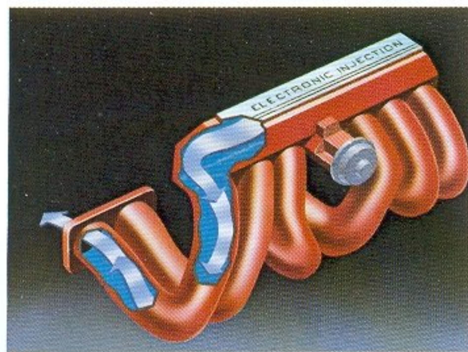
Manifold ram-charged pressure pulses boost torque.
