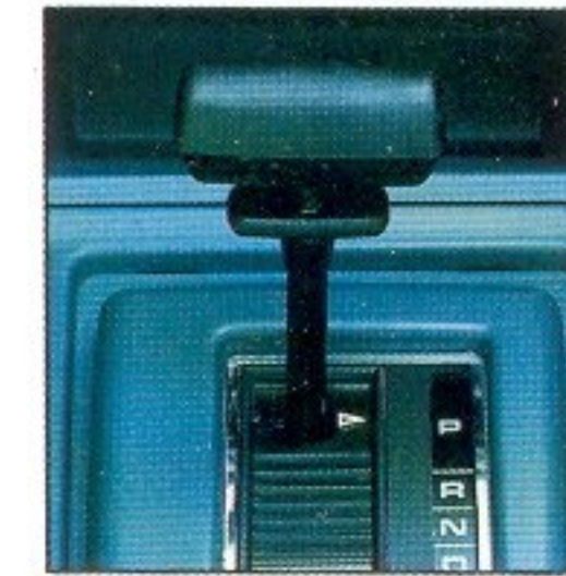
3-speed, floor-shift Trimatic automatic transmission.
