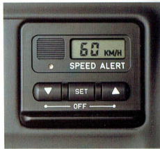
The new speed alert system gives visual and audible warning if the car exceeds your pre-set speed limits. Also, new lamp and chime warning highlights low fuel and car moving with handbrake on.
