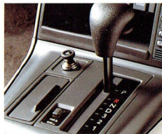
Electronics have created a revolution in transmission technology. In power mode, the driver has later upshifts for more engine power.
