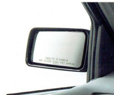
Convex left hand side rear vision mirror helps avoid any blind spots when changing lanes or reversing.
