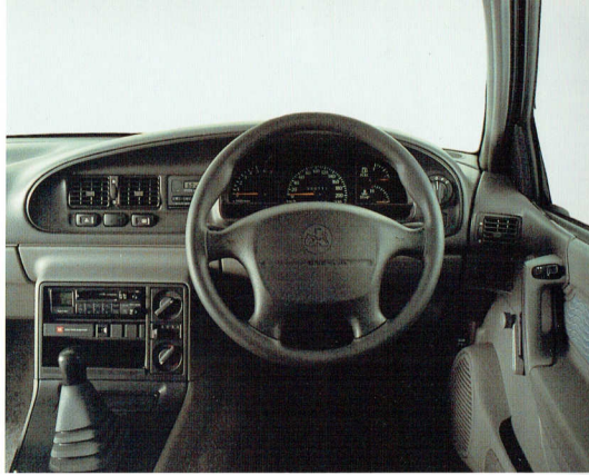
A. The airbag is triggered by a crash sensor, which is a self-contained, electronic sensing, microprocessor-controlled system.
