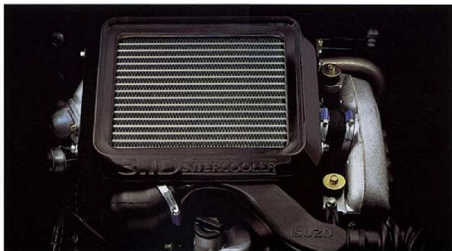
Jackaroo's intercooler is an air to air type which drops the temperature of the inlet air going into the cylinder making it more dense.
