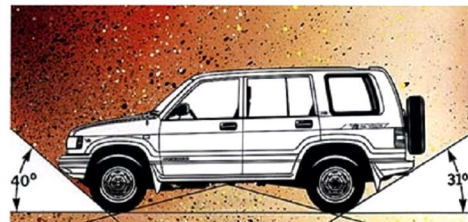
Its intelligent dimensions are best exemplified by its impressive long wheelbase yet relatively short overall length, accounting for the Jackaroo's excellent manoeuvrability. The Jackaroo's approach angle is a stunning 40 degrees with a departure angle of 31 degrees due to its efficient dimensions. The ramp over angle is 21 degrees for the LWB and 24 degrees for the SWB model.
