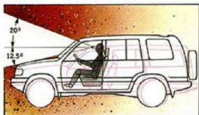
This comparative illustration clearly demonstrates the superior visibility that Jackaroo has over a conventional station wagon.
