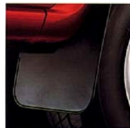
Flexible mud flaps to keep excess mud from forming in wheel arches or flinging stones.
