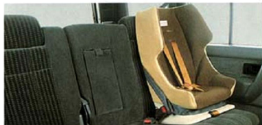
The velour trimmed rear seat comes with retractable headrests, centre armrest and child seat anchor points.
