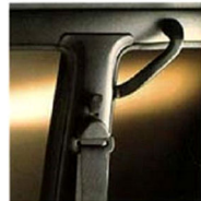
Height adjustable seat belt anchor point on pillar to ensure maximum comfort and safety for all passengers, regardless of height.
