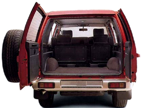
70/30 rear doors open to the left unlike all other 4WDs. So you're not opening a heavy door onto a road when parked. And with Australia's road crown it makes it even less of an effort. The rear door also has a lock to ensure it won't slam shut unexpectedly.
