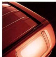
Rear window dust deflector for superior rear visibility (standard on all models).
