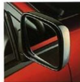
Large electric external mirrors that are heated to keep them clear of moisture. Plus they're electrically retractable via a button on the dash. Ideal for narrow bush tracks or city lanes.
