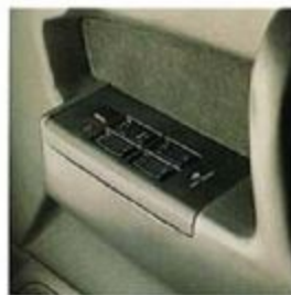
Electric windows and central locking controls are positioned on the driver's door.
