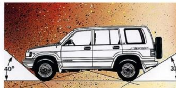
Its intelligent dimensions are best exemplified by its impressive long wheelbase yet relatively short overall length, accounting for the Jackaroo's excellent manoeuvrability. The Jackaroo's approach angle is a stunning 40 degrees with a departure angle of 31 degrees due to its efficient dimensions. The ramp over angle is 21 degrees for the LWB and 24 degrees for the SWB model.
