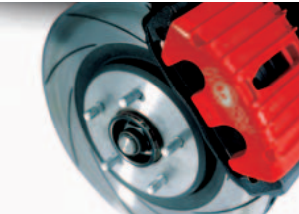
AWD Performance Braking System with massive 336 x 32mm 'AP Racing' ventilated and grooved front discs, HSV-embossed twin piston "Corvette" front calipers in HRT red, 315 x 18mm ventilated and grooved rear discs.
