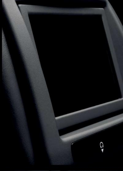
The remote controlled DVD player shows DVDs through LCD screens integrated into the back of the front seat headrests, with sound channelled through stereo headsets.
