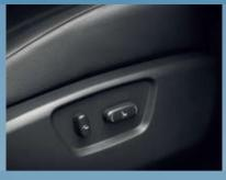
The eight way power driver's seat in Captiva MaXX enables fingertip control of slide and recline adjustment, plus individual height control of the front and rear cushions.
