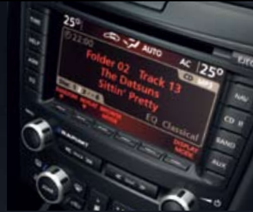
Multifunction colour LCD display The centre console mounted full colour screen displays full audio system details and the dual zone electronic climate control settings for driver and passenger. It also provides full colour mapping when the optional satellite navigation is installed.
