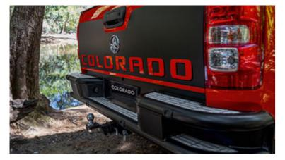
Rear Steel Step, Colorado Decal and Towing Package
