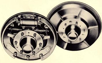
Note the design of the brakes which have self-energizing shoes, reducing the amount of pedal pressure necessary. The brake linings are of extra thickness to give long life, while the shoes are adjustable to take up wear simply by turning two exterior nuts on each brake drum dust shield. The drums are of cast iron ribbed for heat dissipation and to prevent distortion.
