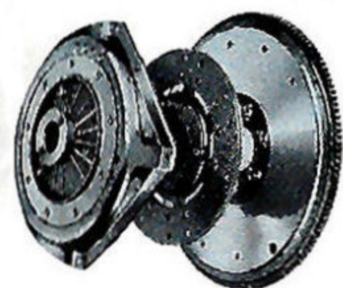
Pontiac's improved easy action clutch is exceptionally smooth in operation and, due to its extremely simple design, has fewer working parts to wear and get out of order, thus assuring long, trouble-free service. The addition of a booster spring to assist in completely depressing the clutch pedal makes it possible to disengage the clutch with scarcely more pressure than the weight of the foot.
