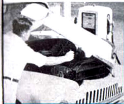
A simple grip-and-twist action unlocks hinge for raising; when closed the mechanism locks to form an easy-acting hinge.
