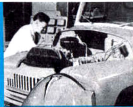
The bonnet is easily removed. "Special" mud-guard design provides extra working space between engine and mudguards.
