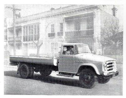
AB-150 series trucks are ideal for either farm or industry. They feature heavy-duty front and rear axles and have straight frame chassis designed to carry heavy loads.
