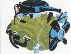
2. Astro-Flame 230 h.p. 327 cu. in. V8. This is the source of the tremendous power of the Pontiac Parisienne Sport Sedan. It obtains its ultra-high performance from special cylinder heads, 4-barrel carburettor, aluminium alloy main and connecting rod bearings, special alloy machined fly wheel, heavy-duty 5-bearing crankshaft, thermostatically-controlled fan. The Astro-Flame features a full-flow oil filter, oilwetted paper element type air cleaner, and hydraulic valve lifters.
