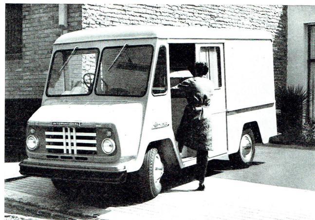
ABM-120 Metro Van with walk-through body.
