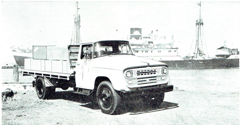
C-1500 fitted with tray body for general cartage.
