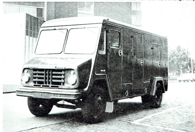
ABM-160 Metro Van fitted out as fire tender.
