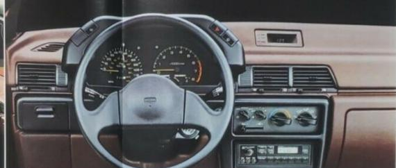
Sporty but practical. The Colt 200 dash blends form and function with large, easy-to-read instruments. (Tachometer not included on E and Dt. 4-doors.) Sensibly laid out switches are easy to use, even at night.
