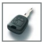
The key for the 206 contains an electronic code for the anti-theft immobiliser, which is recognised when the key is placed in the ignition. If the correct code is not read, the car will be immobilised. The key also activates the locks on all doors including the hatch, using a high-frequency remote control unit. The
