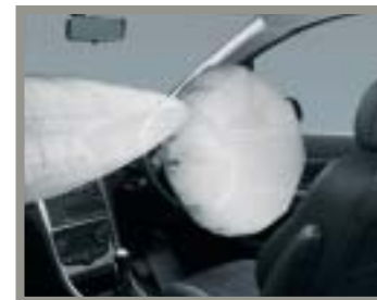
Front, side and curtain airbags - six in all
