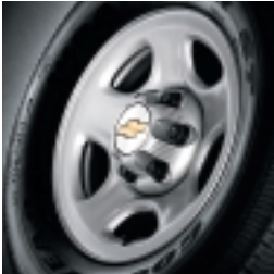
16" PAINTED STYLED-STEEL WHEEL WITH PAINTED CENTER CAP. STANDARD ON ALL BASE MODELS. CHROME CENTER CAP IS STANDARD WITH ALL LS MODELS.
