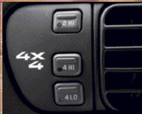
Engage the S-10 Insta-Trac system with the push of a button.
