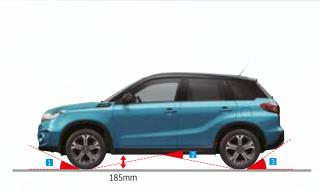
Approach angle: 18.2° Z Ramp breakover angle: 17.7° 3 Departure angle: 28.2°
