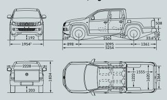
$^14 MOTION\ models\ have\ 192 mm\ minimum\ ground\ clearance\ /\ 2WD\ models\ have\ 230 mm\ minimum\ ground\ clearance\ .^2\ Body\ width\ including\ wheel\ arch\ flares.$
