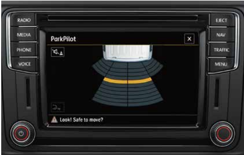
Rear Park Distance Control. Emits audible warnings when obstacles are detected behind the vehicle when parking, and also provides a visual display of the vehicle's distance from the obstacles.
