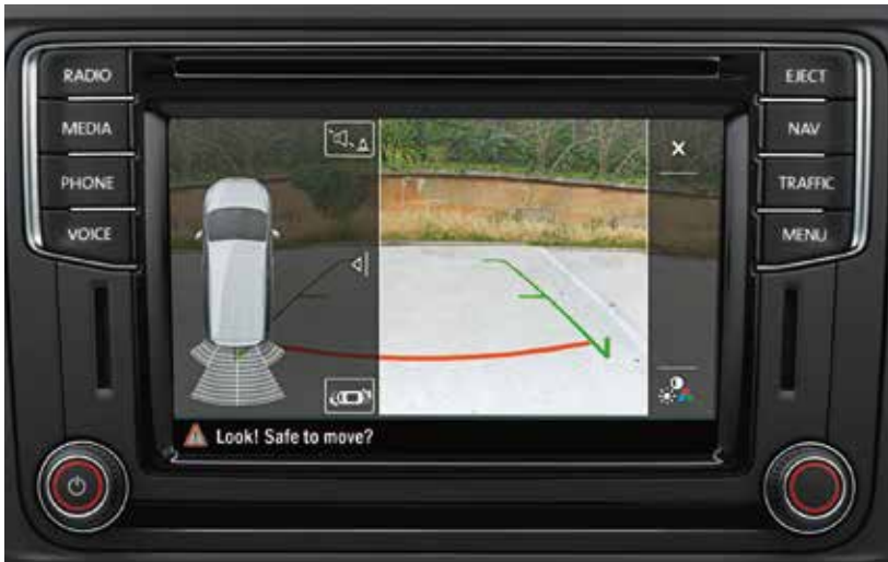
Rear View Camera (RVC). Simplifies parking by showing a limited view of the area behind the vehicle on the display of the radio or navigation system. Additional static guidelines facilitate the parking process. Optional reversing camera only available in conjunction with lifting tailgate.
