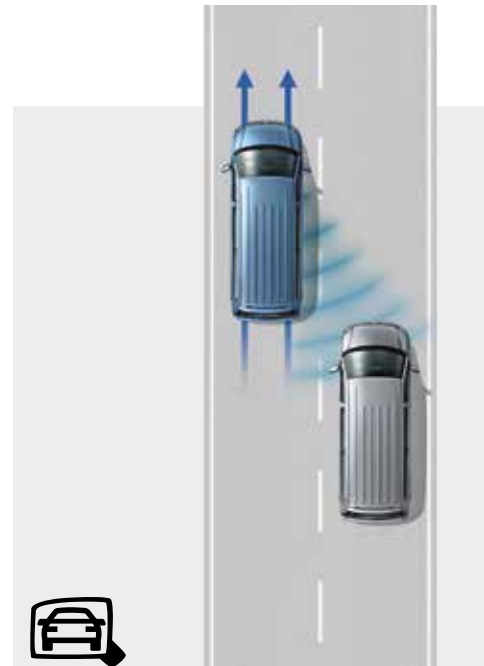
Lane change assist "Side Assist". Displays a warning signal in the door mirror if one of the system's sensors registers a vehicle in the blind spot when changing lanes. Available on Short Wheelbase Van and Crewvan only.
