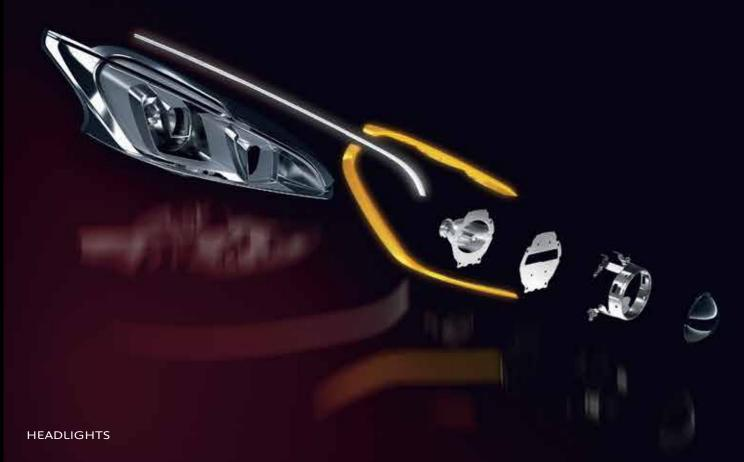
Peugeot 208 GTi has standard halogen headlights with rectangular internal structures and light guides and indicators using LED (Light Emitting Diode) flat-guide technology\*, ensuring maximum lighting and giving the car a strong, stand-out look.
