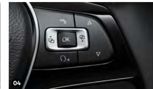
04 Voice Control. You are free to operate the telephone and audio functions without taking your hands off the steering wheel. Furthermore, you can call up virtually all menus and notifications on the radio using voice control. | CE | CE | CE6 | SL | HL | AV |
