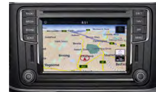
03 Discover Media navigation system. In addition to the functions of the Composition Media radio system with six loud speakers, there is a second integrated SD-card slot which is compatible with the SD-card with the map data. | HL | AV |
