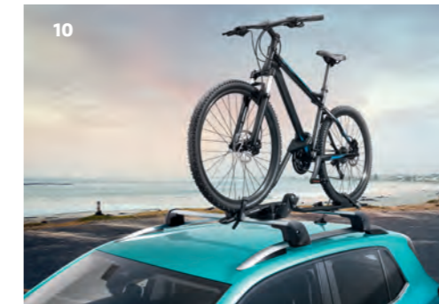
10 Bicycle carrier The aerodynamic bicycle holder has a quick-fastening system that makes it easy to fit and can be locked for piece of mind. Part.no 000071128F
