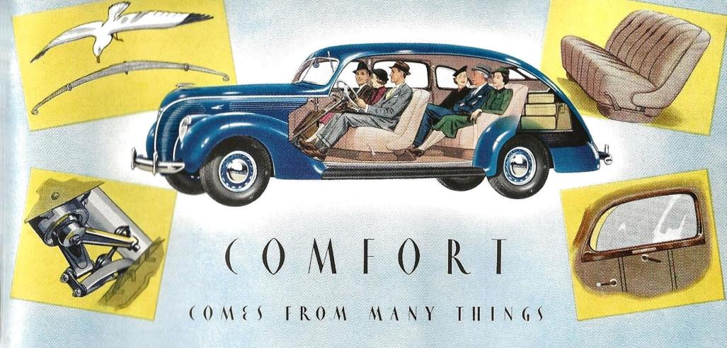
A combination of features, exclusive with Ford in the low-price field, contributes to the luxurious comfort of the 1938 Ford V-8. Foremost is the Ford Center-Poise principle, by which passengers ride near the center of the car, between the axles instead of over them, cradled by flexible transverse springs.
