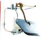
Smooth. Hydraulic clutch control minimises the transfer of engine vibration, giving smoother engagement and an inert' clutch pedal.
