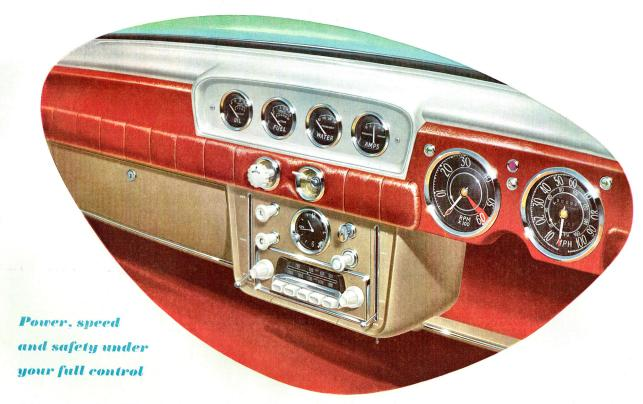
Stylish, compact and beautifully equipped, the control panel of the Sunbeam Rapier is designed for high performance driving. In addition to a speedometer and fuel and oil gauges, the lavish equipment includes as standard: revolution counter, ammeter, thermometer, two-speed wind-screen wipers and cigar lighter.
