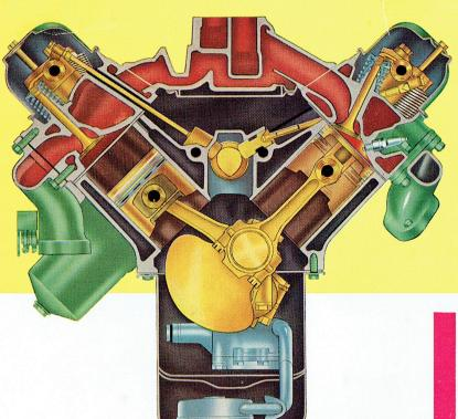
Longer, stronger crankshaft with big main and connecting rod bearings mean less wear and longer bearing life.
