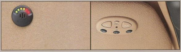
Reverse Parking Sensor A big help when you're backing into tight spots. A sonar-like system alerts you to fixed obstacles in your way when backing up. A speaker and LED display provide audio and visual cues when an object is sensed within 6 ft. (2 m) of the bumper. The beep becomes more frequent and the lights go from green to yellow to red as the object gets closer. A red light and constant beep alert you when an object is 10" (2.5 cm) away. Dealer installation recommended. Available for LS.
