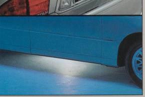
Underbody Security Lighting With underbody security lighting, you'll never have to approach a dark vehicle again. This system provides light to the underside of the vehicle using two powerful lights mounted under the vehicle. The system automatically lights up when you use your keyless entry key fob or manually unlock the doors. Available for Blackwood, Navigator and Town Car.
