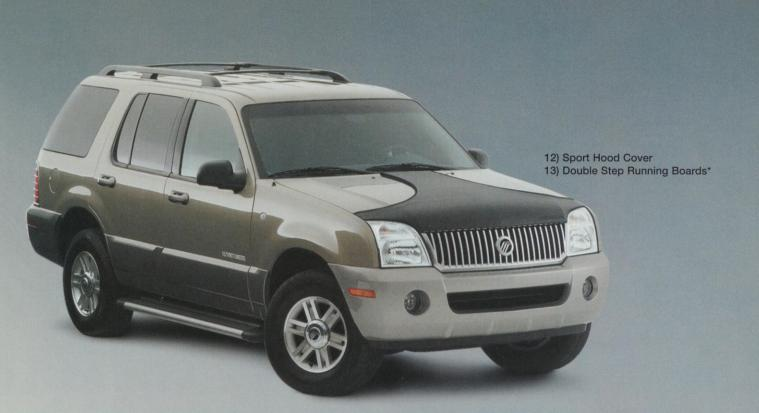
**12) Sport Hood Cover** Add a sporty, stylish look to your vehicle while helping to protect the hood's finish from bugs, stones, salt and road debris. Constructed of a heavy-duty vinyl with a flannel backing. One-piece design allows hood to be opened without removing cover. **Available for Mountaineer**.
