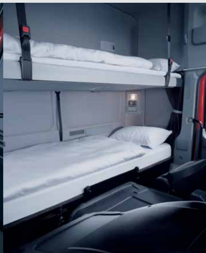
Plank beds are a thing of the past: below the 64.5 cm wide standard bed for L-cabs, above the optional 70 cm wide luxury bed for L-cabs with raised roof.
