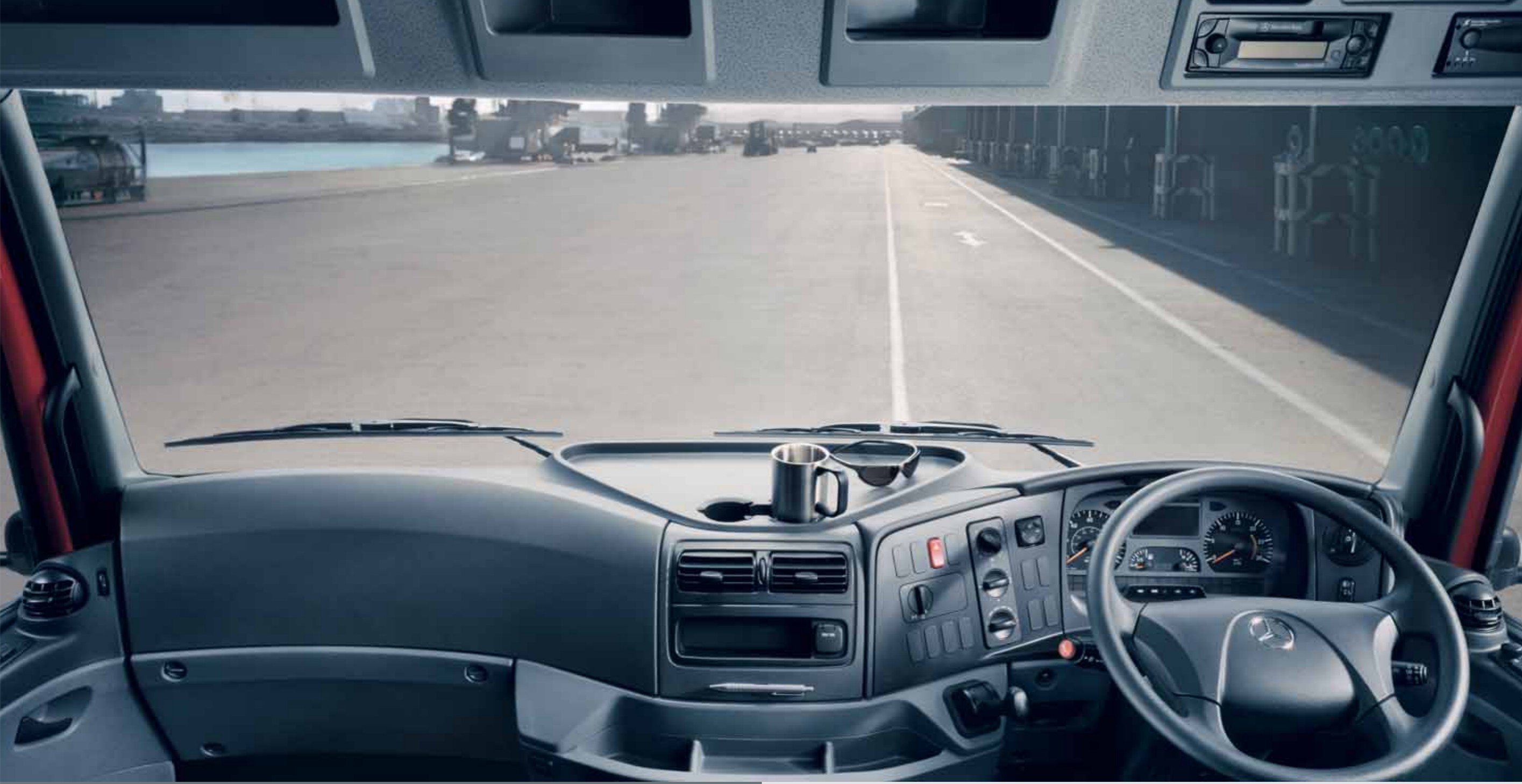
Acceleration and braking: a single control stalk is used to operate the cruise control and engine brake functions.
