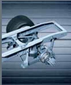
The 4x2 prime-movers with an air-sprung rear axle are fitted with 2-bellows air suspension which makes for more stable handling qualities and improved driving dynamics.
