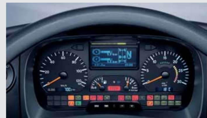
The anti-glare instrument cluster: the function check covers the most important vehicle data and functions and, apart from the tyre checks, assists the daily exterior checks of the vehicle carried out by the driver.
