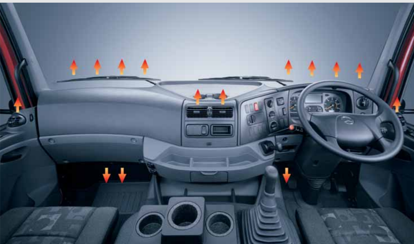
The new air-controlled heating system can be individually adjusted and distributes the air through a cleverly thought-out system of air ducts and outlet nozzles. It has a fast response time and thus reacts quickly to driver inputs.
