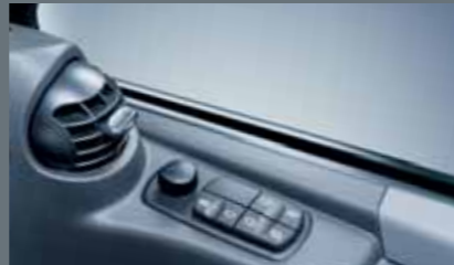
The new door operating panel with easy-to-use function buttons: for adjusting the exterior mirrors on the driver's and co-driver's side, switching the exterior mirror heaters on/off, operating the power windows on the driver's and co-driver's side and - as an option - activating the central locking or extended central locking system.
