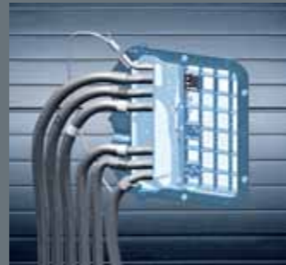
Simple connections without tiresome cable routing: the new body manufacturer interface integrated centrally in the cab hatch simplifies communication between the cab and the body and affords the body manufacturer easier access to the electrical systems.
