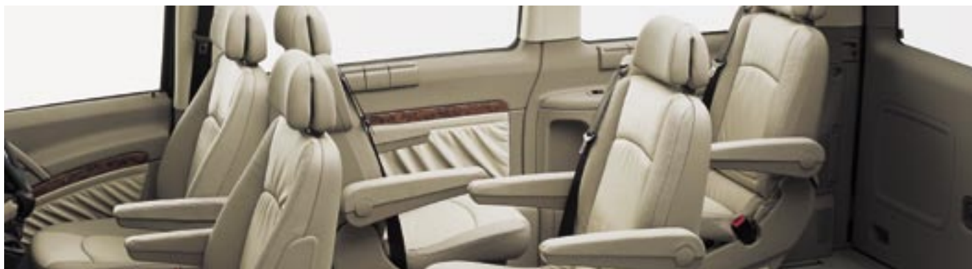
The seats in the Viano can be adjusted easily in increments of 25 mm
