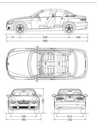
All dimensions of the technical drawings in millimetres. Luggage compartment capacity (VDA method): 210-350 litres.
