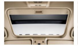
□ **Glass sliding/vent roof,** electric, with wind deflector and comfort opening function via the car's remote control unit.
