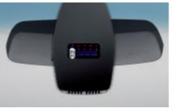
■ Rain sensor with automatic headlight activation: Once activated, the rain sensor will automatically switch on the windscreen wipers when it begins to rain, adjusting the wiper frequency in line with rainfall intensity. The integrated automatic headlight activation system will switch on the low beam automatically at dusk and in tunnels.
