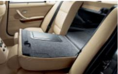
□ **Through-loading system** with asymmetric 60/40-split folding backrest and ski bag (standard on 323i, 325i and 330i).
