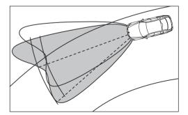
□ The Adaptive Headlights system features electromechanically controlled headlights to ensure optimised road illumination as soon as the vehicle enters a bend. This enhances safety when driving at night or in bad visibility. Sensors register the steering angle, yaw rate and vehicle speed; the direction of the headlight beams is then automatically adjusted to match the calculated layout of the bend (standard on 330i).
