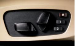
□ Seat adjustment, electric, for driver and front passenger, with electric adjustment of seat height, backrest, fore/aft position and seat angle, plus memory function for driver's seat and exterior mirrors (incl. automatic tilt function). Two personalised settings can be stored for the driver's seat and the exterior mirrors (standard on 325i and 330i).
