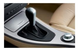
□ **6-speed automatic transmission** with Steptronic. The gearshift mechanism enables very fast, immaculate gear changes – for truly dynamic performance(standard on 320d, 320d Executive and 330i).
