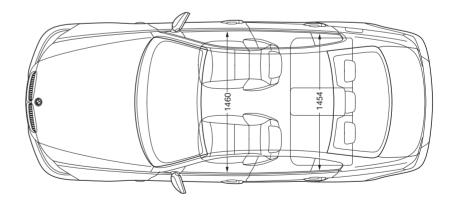
All dimensions in millimetres. Luggage compartment capacity (as per VDA standard): 460 litres.
