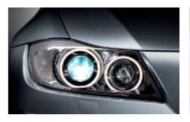
□ Xenon headlights for low and high beam, including four parking light rings and automatic headlight range control, provide improved illumination of the road ahead at night or in poor visibility (standard on 330i).
