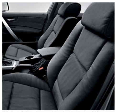
□ **Comfort seat** for driver and passenger, with draped pockets, electronic seat height and backrest angle adjustment, length adjustment and tilt control, as well as memory function for driver seat and wing mirror (automatic mirror down-tilt). Additional electr. adjusting functions: variable shoulder supports and headrest.
