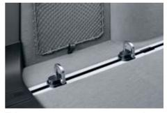
■ Storage compartment package with front armrest, luggage nets behind the front seats, under centre console on the passenger side and on the left side of the luggage compartment; reversible luggage compartment floor and parcel rails with four fastening eyelets (illustrated).
