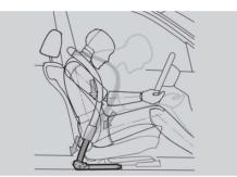
■ BMW restraint system for the driver and front passenger consists of a combination of the three-point seat belt, belt tensioner and belt force governor. For optimum restraint in a collision.
