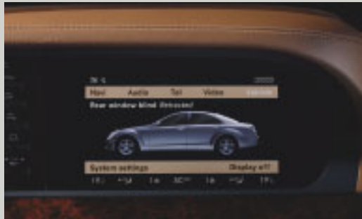
COMAND display The COMAND display is positioned next to the instrument cluster, directly in the driver's line of view
