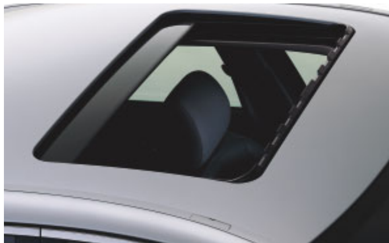
Tilting/sliding glass sunroof, electric, with PRE-SAFE® closing function
