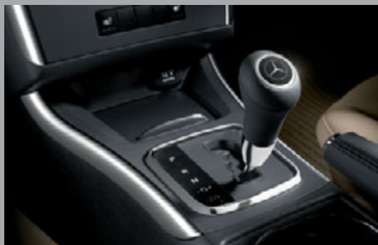
The selector lever of the CVT automatic transmission
