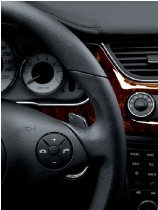
Shift paddles on the steering wheel put sporty gearchanges at the driver's fingertips
