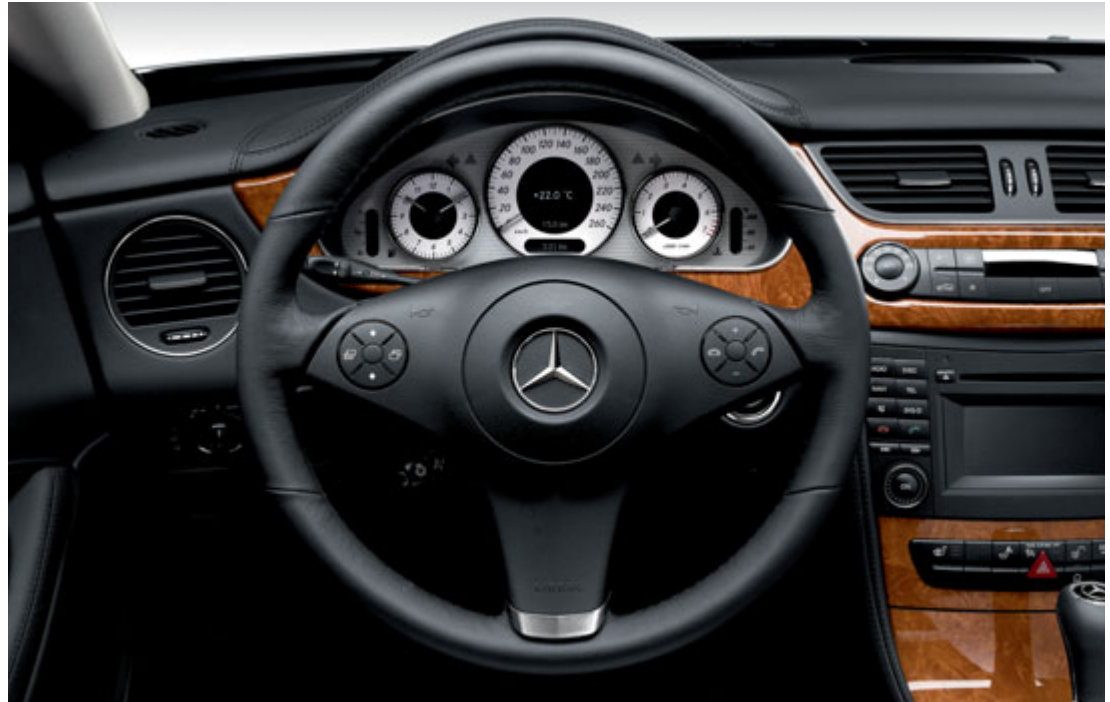
The multifunction steering wheel allows the driver to use the telephone and the radio as well as to select various vehicle functions which are shown on the instrument cluster display while keeping both hands on the wheel
