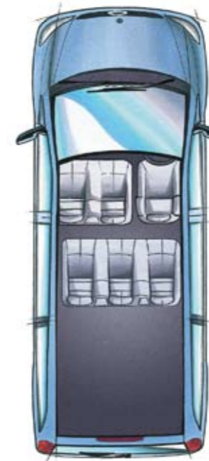
The back row of seats can be removed to create more luggage space.
