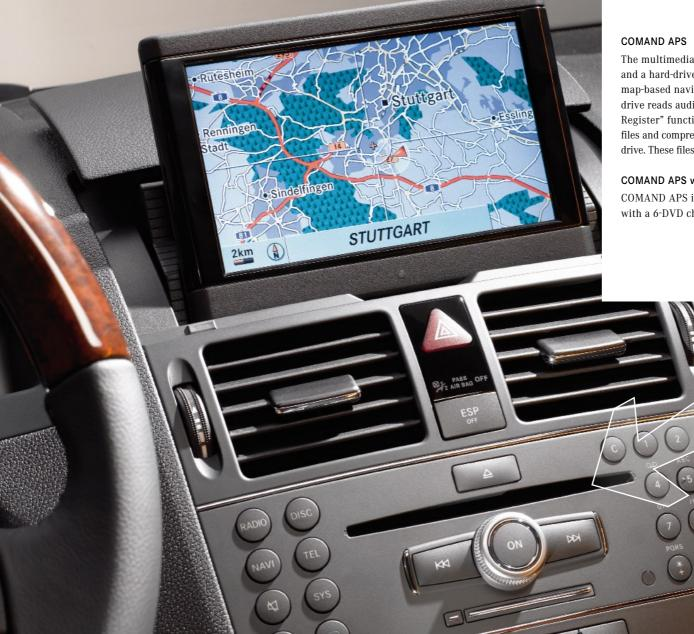
The multimedia system features a fold-out 7" colour display and a hard-drive navigation system for fast, high-resolution map-based navigation throughout Europe. The integral DVD drive reads audio CDs/DVDs and video DVDs. The "Music Register" function allows the user to copy and save music files and compressed audio files (e.g. MP3) to a 4 GB hard drive. These files can be imported from CD, DVD or memory card
