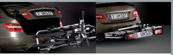
The laden bicycle rack can be pivoted downwards, allowing the boot to be opened
