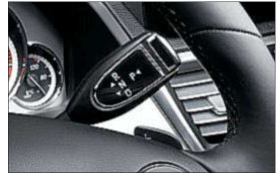
Transmission for the V6 and V8 engine variants operated at the push of a button using the DIRECT SELECT lever on the steering wheel
