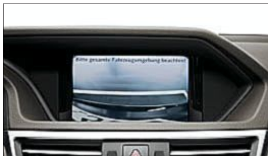
The reversing camera's wide-angle lens films the area directly around the rear of the car
