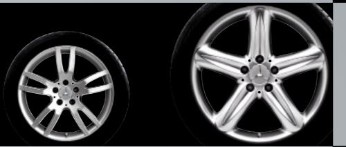
On all light-alloy wheels, use wheel bolt A211 401 0370 and the corresponding rim lock B6 647 0144 (from spring 2008: B6 647 0155). Light-alloy wheels are supplied without tyres, wheel bolts
