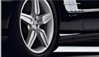
Tarka | 5-spoke wheel Incenio designer wheel | Finish: sterling silver Wheel: 8.5 J x 19 ET 35 | Tyre: 255/35 R19 Option for rear axle: Wheel: 9.5 J x 19 ET 40 | Tyre: 285/30 R19
