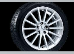
18" AMG multi-spoke wheel | Style V AMG light-alloy wheel Finish: high-sheen Wheel: 8.5 J x 18 ET 30 | Tyre: 255/40 R18 Option for rear axle: Wheel: 9.5 J x 18 ET 33 | Tyre: 285/35 R18
