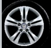
**5-twin-spoke wheel** Finish: titanium silver Wheel: 8.5 J x 17 ET 35 Tyre: 255/45 R17
