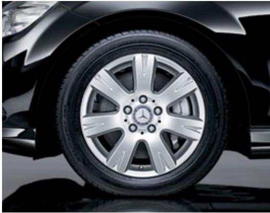
7-spoke light-alloy wheel with 205/55 R 16 tyres
