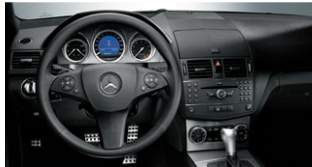
Behind the 3-spoke nappa leather steering wheel are shift paddles for manual gear changes (in conjunction with automatic transmission)
