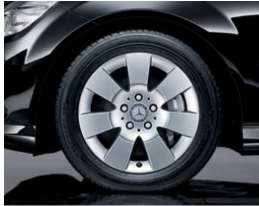
7-spoke light-alloy wheel with 225/50 R 16 tyres
