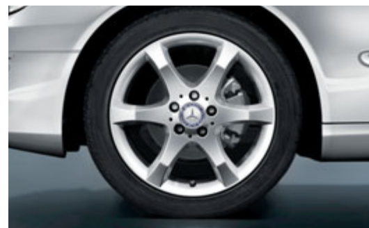
Optional extra: 6-spoke light-alloy wheel with 225/45 R 17 tyres at the front and 245/40 R 17 tyres at the rear
