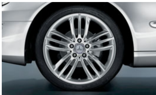
Accessory wheel ex factory: incenio 5-triple-spoke "Korsunia" light-alloy wheel with 225/40 R 18 tyres at the front and 245/35 R 18 tyres at the rear
