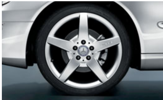
Optional extra: AMG 5-spoke light-alloy wheel with 225/40 R 18 tyres at the front and 245/35 R 18 tyres at the rear
