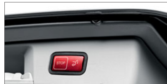
You can also open and close the EASY-PACK tailgate in a low position at the push of a button
