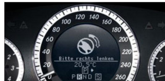
Parking Guidance indicates suitable parking spaces to the driver and provides parking directions
