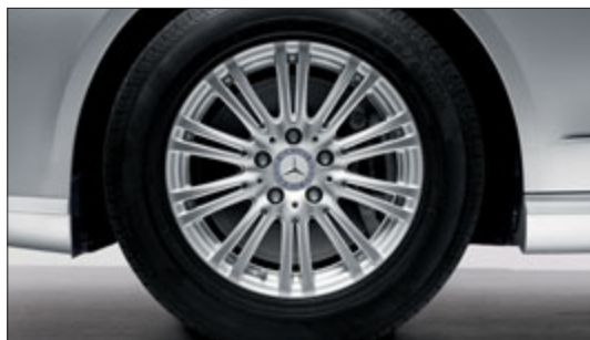
10-twin-spoke light-alloy wheels with 225/55 R 16 (standard for ELEGANCE) or 245/45 R 17 tyres (optional, standard for E 500 and 4MATIC models)
