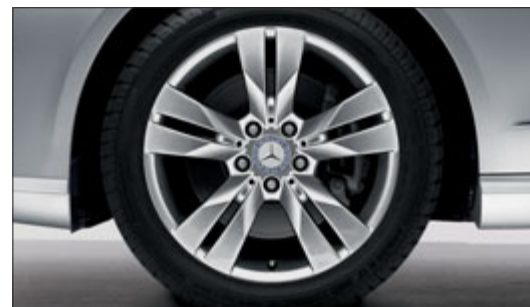
5-twin-spoke light-alloy wheels with 225/55 R 16 or 245/45 R 17 tyres, high-sheen finish (optional extra, Code R 78 or R 48)
