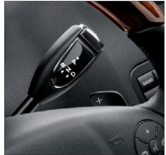
DIRECT SELECT steering-wheel shift paddles and selector lever
