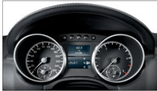
The tubes in the instrument cluster feature chrome rings and white needles with a 3D scale
