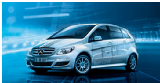
The B-Class F-CELL is locally emission-free thanks to an electric drive system which draws its energy from a fuel cell
