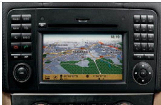
COMAND APS integrates information, communication and navigation in a single system
